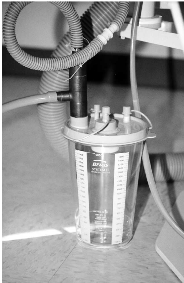
Fig. 1. Apparatus used to collect chair side wastewater samples.
