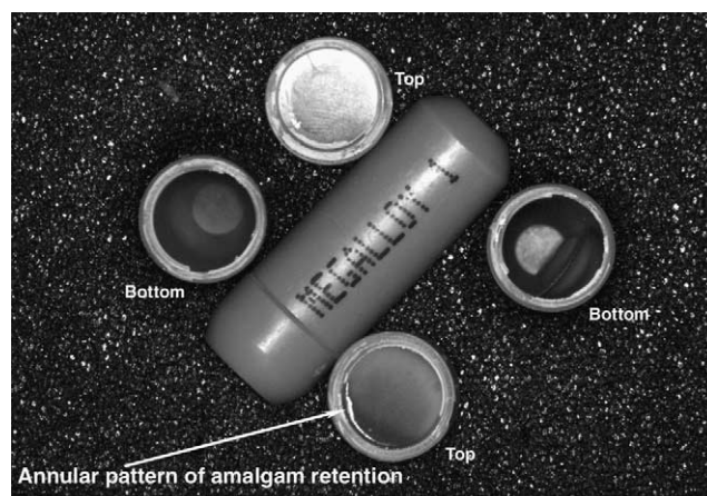
Fig. 1. Photograph of one ultrasonically sealed Megalloy™ capsule and two capsules triturated and opened. Arrow identifies an annular pattern of retained amalgam in the top portion of one of the amalgam capsules. This pattern of amalgam retention was seen in virtually all the ultrasonically sealed capsules used in this study.
